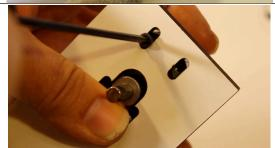
Put a hex nut in the slot on the back of the small drive gear and screw a M3x10 into it just enough to catch a few
