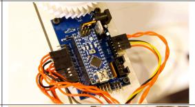
Put the crimps for two wires into a 2x1 housing, and plug it in to the headers marked Motor. Cut the wires to the length needed to reach the motor and strip the ends. Hook the bare wire through the motor terminals and tack them down with some solder. It doesn't matter which terminal the wires go to. If the motor turns the wrong direction, plug it in with the other wire on +.
