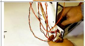
Plug R into Guide Min, L into Guide Max, C into Sensor Cal, A into Auto. Plug the servo into Servo with the brown wire at the bottom. Plug P into PWR on the right side of the board and plug the potentiometer into Knob. If, when first operating the winder you find the knob is working backwards, flip the plug over.
