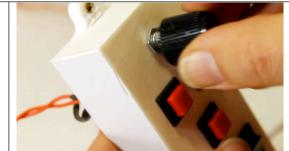
Mount the control box to the base with two M3x16 screws. You can run the wires through the hole under the base, or up through the notch next to the box to run them over the base if preferred.
