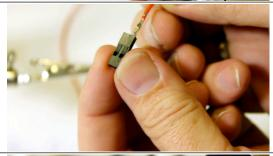
You can quickly twist the wires by lightly chucking the housing into a drill and spinning it.
