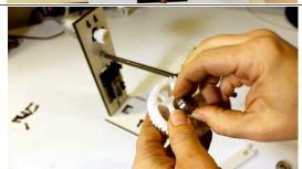
Put the magnet on the table and flick it a few times so it spins freely and is able to orient itself to the earth's magnetic field. Make note of the face that points north, perhaps coloring it with a marker. Place the magnet in the small hole on the flat side of the spool gear with the marked pole facing outward. Don't glue the magnet in until you have tested it and are certain the correct pole faces outward.
