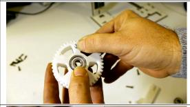
Slide the spool gear onto the rod. Note that if you plan to use a spool with a 80mm hub you may need to add a washer between the nut and the spool gear to keep the spool from catching on the electronics. Loosen the motor screws so it can slide down to engage the drive gear with the spool gear. Adjust the position of the drive gear on the motor shaft to line them up if necessary. Tighten the motor screws.
