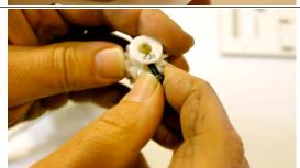
Slide the drive gear on to the motor shaft with the nut facing the motor and positioned over the flat of the shaft. Tighten the screw the rest of the way so that it just contacts the flat of the shaft. If you over tighten, once the screw can't go any further through the nut, the nut will instead rise up and break out of its slot.
