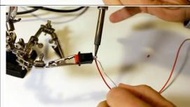
For the potentiometer, use one color for the left and right pins and a different color for the middle pin. Attach the wires with a dab of solder, keeping the iron in contact for as short a time as possible. It is possible to overheat the potentiometer and ruin it, so if the solder doesn't melt on contact with the tip, take the iron away and wait a few seconds before trying again.
