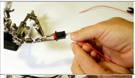
Put a dab of solder on the wire to secure it to the terminal. You can choose to use different colored wires for each terminal, but the polarity doesn't matter. Do the same for the each of the other buttons and switches
