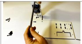
Put a finger under the nut trap and drop a square nut into it. Slide a M3x25 screw through the hole at the bottom of the base into the slot, and thread it through the square nut. Tighten it just enough to be secure. Over tightening could crack the wood.
