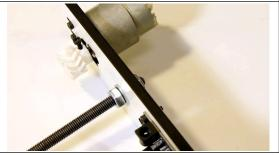
Slide the tabs on the bottom of the motor mount into the slots at the side of the base. It will be a very tight fit, but applying steady pressure and a little sideways rocking will get it to slide in.
