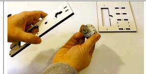
Use two M3x10 screws through the slots to secure the motor.
