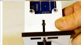
Put bearings into the front and back holes of the spool gear.
